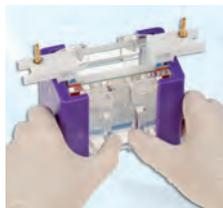
Insert glass plates into PAGE insert and slide clamps into side cheeks to create an effective seal to prevent current leakage during electrophoresis
