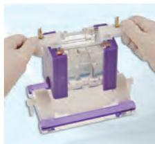
Transfer PAGE insert to casting base, insert cams and turn until tightened
