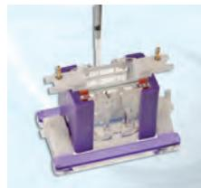
Pour in gel solution, insert comb and allow to polymerise
