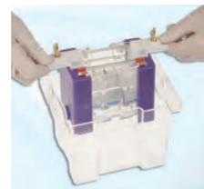
Transfer PAGE insert to tank, fill with buffer, load samples, replace lid and run
